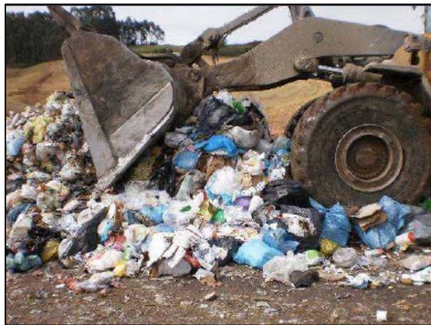
Image 2: Homogenising waste using a loader.
